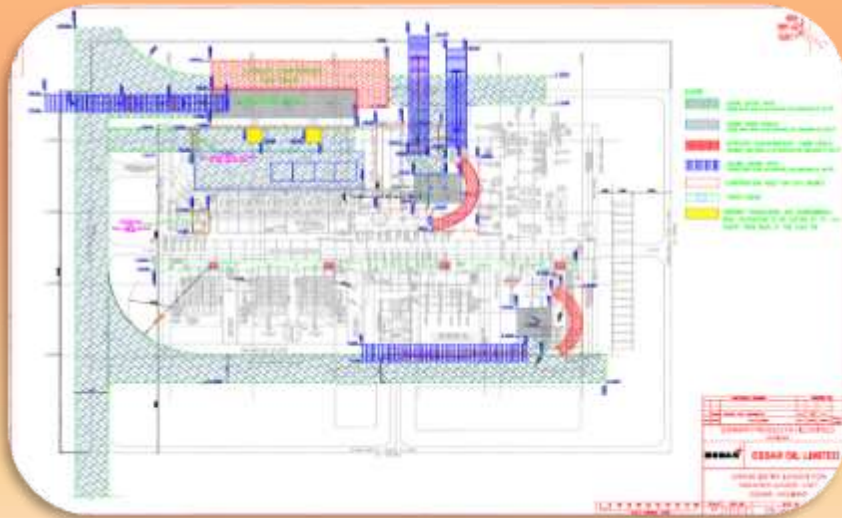
PLAN VIEW OF HEAVY CARGO MOVEMENT AND CRANE LOCATIONS INDICATING STRATA PREPARATIONS & POSITIONINGS
